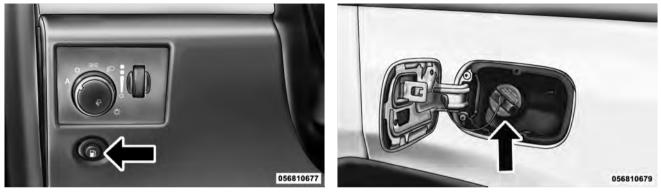
**Fuel Filler Door Release Switch** 2. Open the fuel filler door, and remove the fuel filler
